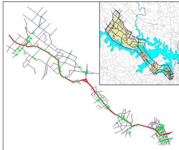
Figure 2. Victoria corridor sub-network. Green points show signals equipped with SCATS count detectors (measured traffic data). Red line demonstrates the main Victoria corridor.
